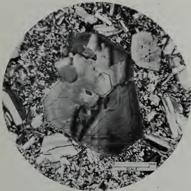
Photo 8. Basalt of Plush Ronch member four showing lobradorite with strong oscillatory zoning and well-developed {100} pinacoids. Section of grain cut parallel to side pinacoid. Crossed nicols.
